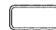
M4 - 9N [30" x 12" MIN.] (2.5 S.F.) (SIZE WILL VARY WITH LENGTH OF STREET NAME) STREET NAME SIGN TO BE USED IN CONJUNCTION WITH M4 - 9 SIGNS BLACK ON ORANGE
