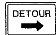
M4 - 9L (LEFT) [30" x 24"] M4 - 9R (RIGHT) [30" x 24"] (5 S.F.) M4 - 9 (L or R) (S) [48" x 36"] (12 S.F.)
